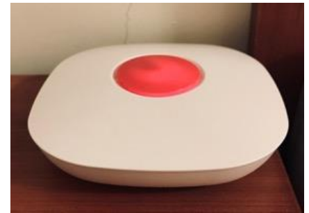
Hardware-indoor type (also outdoor waterproof / explosion-proof type) Optional: UWB / LoRa or UWB / NB-IOT 120 * 120 * 50 (mm)
